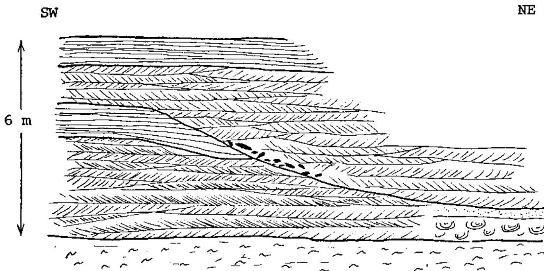
Figure 57. Channel margin at the base of an AB kindred in facies association 1, member 4, Nyborg Formation, between Larsholmen and Innerelv (locality L-17, fig. 69). The underlying silty-sandstone is the top of member 3. No vertical exaggeration.
